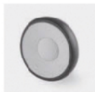
Wheel: XSP electric conductive, non-marking Wheel centre: Polyamide, Tread: Polyurethane, precision ball bearing
